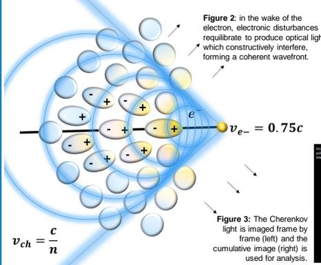
In the context of radiotherapy, Cherenkov light is emitted in dielectric (polarizable) media (e.g. water in the patient), when an incoming, MV x-ray photon ionizes an electron, leaving it with enough energy to travel faster than the phase velocity of light in the medium (Figure 2). Imaging light at these low intensities involves time-gating the exposure around the Cherenkov emission using the linac pulses (Fig. 3).
